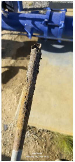
well site electrical conduit rusted through shorting out the wiring, causing no lights or outlets to work inside cargo container.
